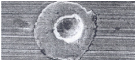
Crater occasioned by electroerosion on the inner raceway of the bearing
